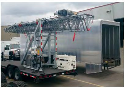
EMU—Emergency Mobile Unit—increases overall network redundancy and further enhances E-Comm's service level to our radio partners. EMU weighs 8,100 kilograms, is more than 30 metres high, and further strengthens the network's backup coverage in the unlikely event of a radio site outage.
